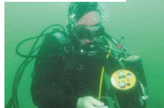
ACTIUM: an underwater location marker for divers, devised by the start-up IANIRA and designed by ENSTA Bretagne research engineers.
