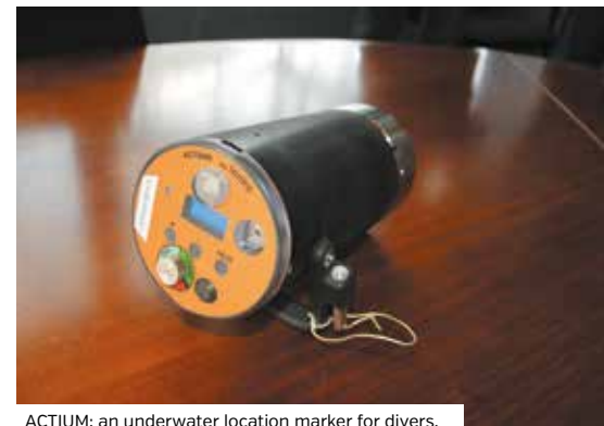
ACTIUM: an underwater location marker for divers, devised by the start-up IANIRA and designed by ENSTA Bretagne research engineers.
